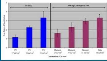
For each energy input, UV and photocatalysis achieved similar levels of adenovirus inactivation. Photocatalysis coupled with filtration exceeded the detection limit of the ICC-qPCR assay.
