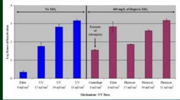
For similar energy inputs, UV and photocatalysis achieved similar levels of inactivation for PRD1. Due to a high level of adsorption, physical removal increased significantly after the addition of TiO<sub>2</sub>.
