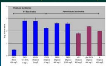
The Photo-Cat achieved rapid viral inactivation—comparable to UV disinfection—even at high TiO<sub>2</sub> concentrations. High TiO<sub>2</sub> concentrations are more effective for chemical destruction.
