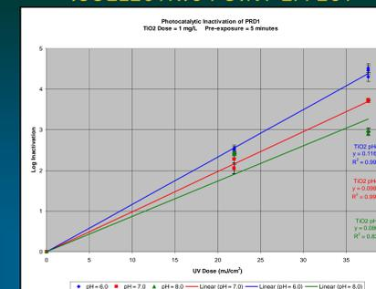
The isoelectric point of TiO<sub>2</sub> is approximately 6.3. At a pH of 6.0, positively charged TiO<sub>2</sub> will be attracted to the negatively charged bacteriophages, thereby increasing the exposure of the bacteriophages to surface hydroxyl radicals.
