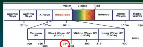
The monochromatic output (254 nm) of low-pressure UV bulbs is the most effective wavelength for disinfection purposes. Conversely, medium-pressure UV bulbs emit light over a wide range of wavelengths but at much higher intensities. Black-light bulbs (350-400 nm), which have been used in similar photocatalysis studies, are capable of activating TiO<sub>2</sub>, but they are not sufficient for disinfection in water and wastewater treatment.
