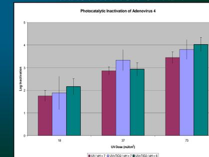
This graph illustrates the differences between the UV and UV/TiO<sub>2</sub> samples after calculating inactivation using the ICC-qPCR method.
