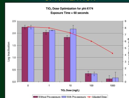
As the TiO<sub>2</sub> dose increases, the water becomes increasingly cloudy—approaching the color of milk—and inactivation decreases significantly. As a result, 1 mg/L was selected as the optimal dose to minimize light scattering and reflection.
