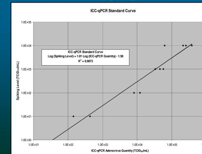
The ICC-qPCR standard curve can be used to calculate the original number of infectious adenoviruses in unknown samples.
