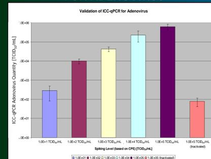
The ICC-qPCR validation graph illustrates the differences between the infectious spiking levels and the inactivation control.
