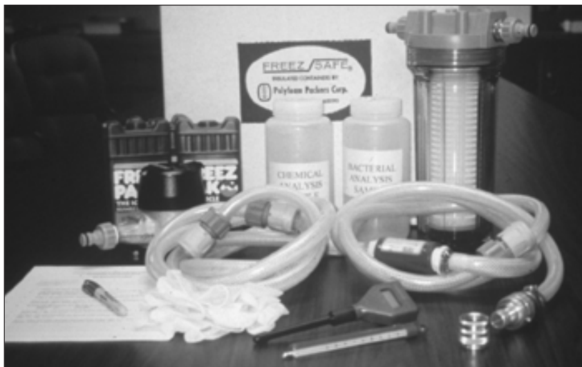
To ensure consistent sampling procedures, 30 identical sample kits were assembled. Each contained all of the equipment needed to collect a sample, along with a flowmeter and an inline flow-restricting device. A 10-min video was also included to demonstrate all of the details of the procedure to further provide for consistency.
